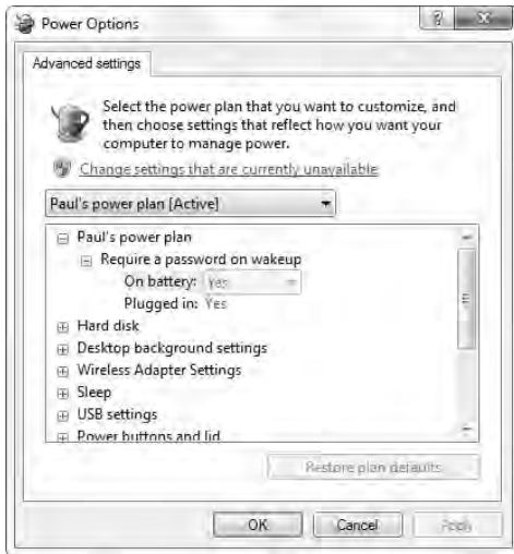
Figure 17-14: Use this rather complicated dialog to handcraft your power plan using every single power management option available to Windows 7.
