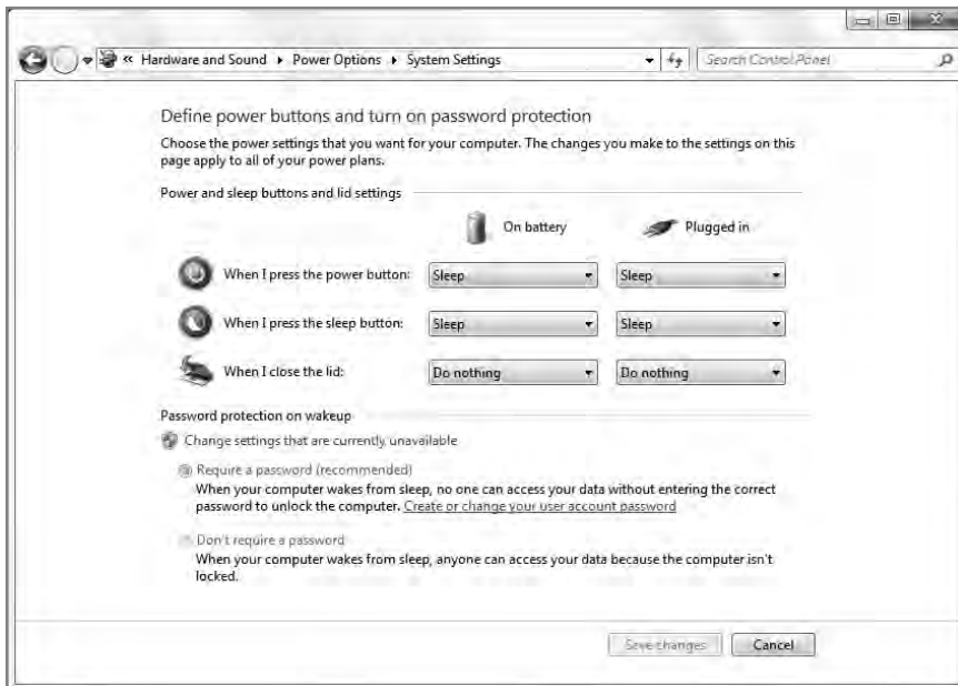
Figure 17-10: Notebook computers and other mobile PCs offer power management options related to the lid and other hardware features.
